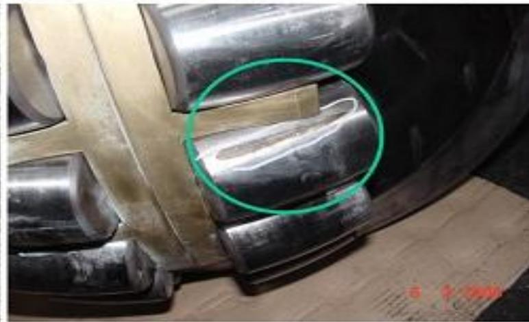
**Exemplary local damages in gears and bearings**
